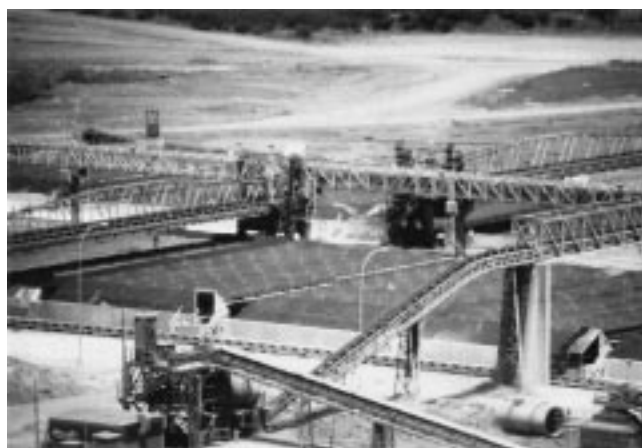
Figure 2 Irrigation of heaps of copper ore at a mine near Santiago, Chile. The crushed ore is stacked on pads and sprayed with a raffinate leaching solution (8 g sulfuric acid plus 0.3–0.5 g residual copper per L) through a system of pipes and nozzles placed on top of the ore. (By kind permission of EM Domic, Sociedad Minera Pudahuel Ltd, Santiago, Chile.)
